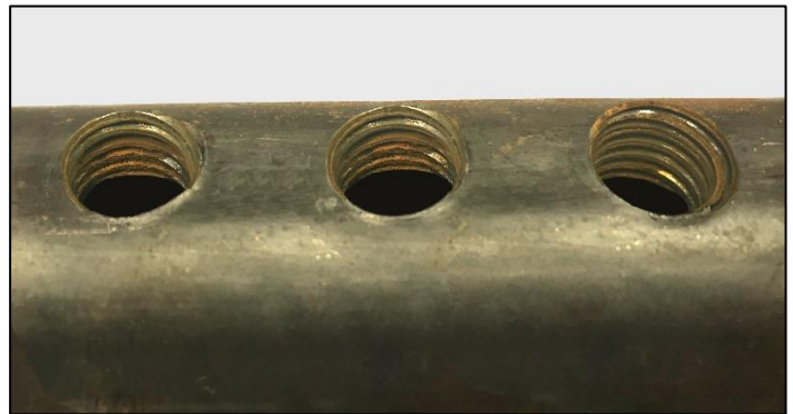
FIGURE 6: Unacceptable Rust in Coupler Threads
