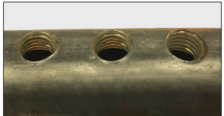
FIGURE 6: Unacceptable Rust in Coupler Threads
