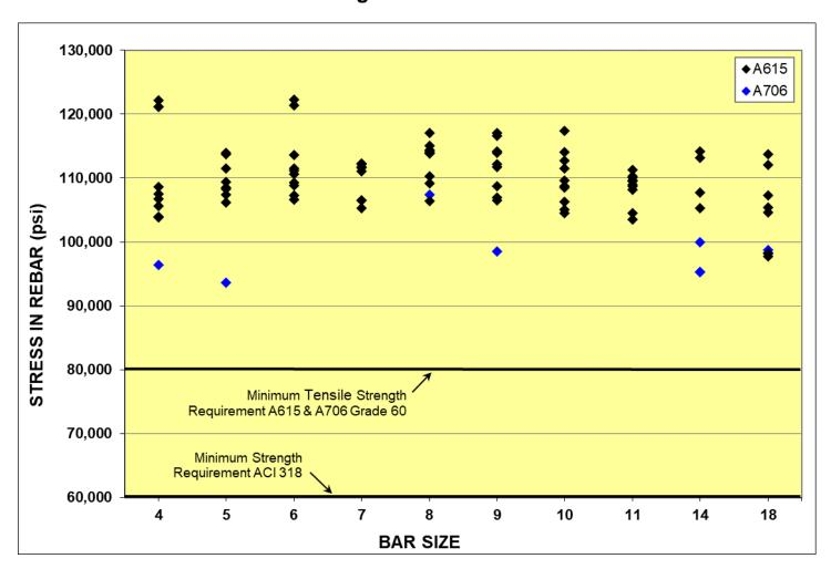
CHART 1: TTGT DoughNUT<sup>™</sup> TENSILE TEST RESULTS
