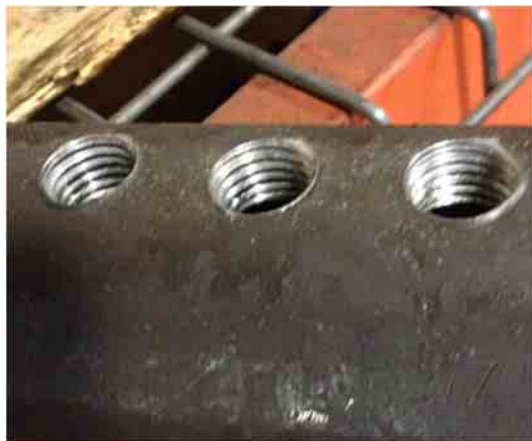
Figure 5. Clean Acceptable Coupler
