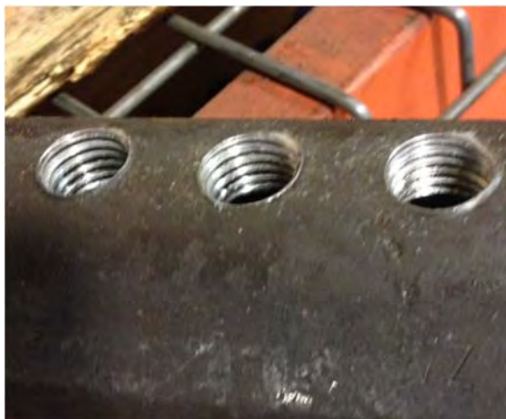
Figure 5. Clean Acceptable Coupler
