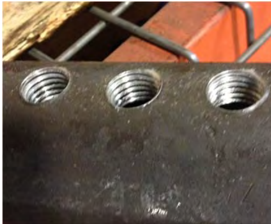
Figure 5. Clean Acceptable Coupler
