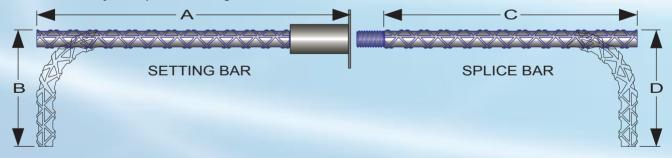
The following chart is an easy way to organize your BPI Barsplicer requirements. Many other configurations can be ordered as shown on the BPI Barsplicer configuration chart... just include the BPI PART NUMBER for easy reference.
