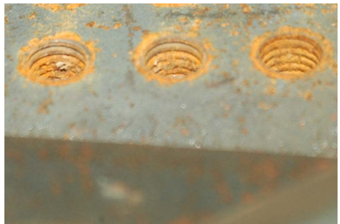
Figure 6. Unacceptable Rust in Coupler Threads
