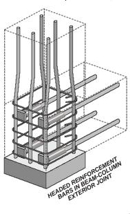
There are many situations in which the amount of space available is not sufficient to fully develop or anchor straight reinforcing bars subjected to tension. In the past, the most commonly used technique to reduce the required development length of bars subjected to tension was to terminate the bars using a 90 or 180 degree hook.
