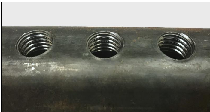
FIGURE 5: Clean Acceptable Coupler
