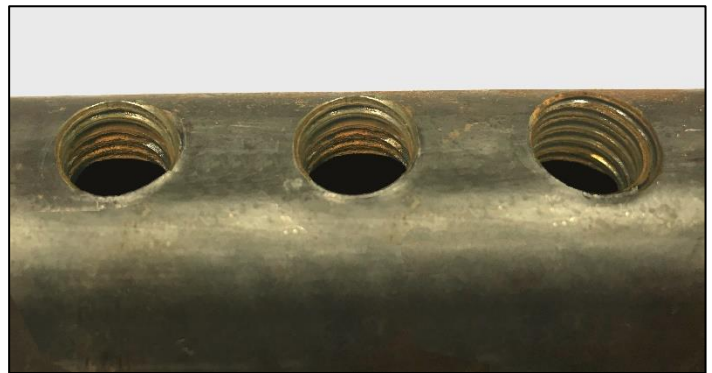
FIGURE 6: Unacceptable Rust in Coupler Threads
