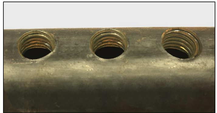
FIGURE 6: Unacceptable Rust in Connector Threads
