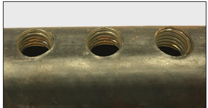
FIGURE 6: Unacceptable Rust in Connector Threads
