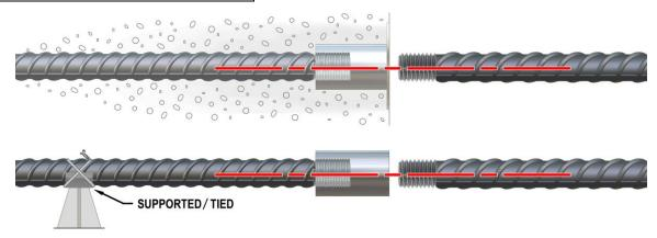
NOTE: If the threaded rebar and coupler threads do not properly engage during assembly, stop immediately. Disassemble the connection to determine the problem. Possible causes of mis-assembly may be mis-matched thread sizes, contaminated threads (i.e. concrete, dirt, etc.) or damaged threads. Re-assemble only after the problem has been identified and corrected.
