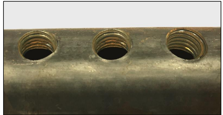
FIGURE 6: Unacceptable Rust in Coupler Threads
