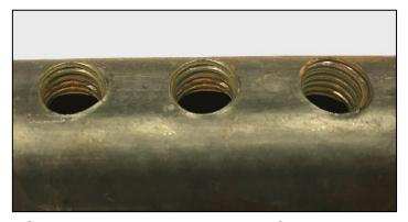
FIGURE 6: **Unacceptable** Rust in Coupler Threads
