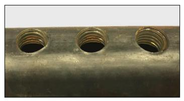
FIGURE 6: **Unacceptable** Rust in Coupler Threads
