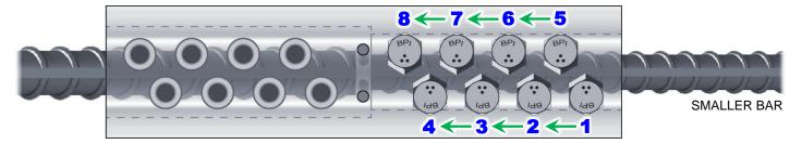
FIGURE 4. Correct Tightening Order, 2<sup>nd</sup> Side (#14 Transitions shown, #18 similar)
