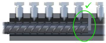
FIGURE 1: Correct Rebar Insertion Depth
