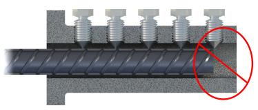
FIGURE 4: Incorrect Rebar Insertion Class HA
