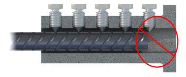
FIGURE 3: Incorrect Rebar Insertion Class A
