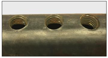
FIGURE 8: **Unacceptable** Rust in Threads
